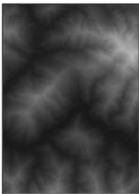
(a) Part of a DTM generated from contour lines (Source: Survey Department)
